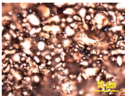
Fig. 5-1 Micrographs of 17-4PH stainless steel powder (average size 11\mu\text{m} ) used in the subsequent tests, observed by optical microscope.
