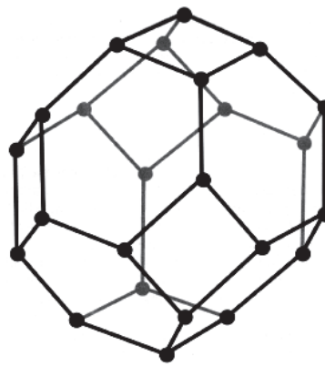
Fig. 4-9 The isolated spherical pores located at the corners of boundaries of tetrakaidecahedron grains in the final stage of sintering [24] .
