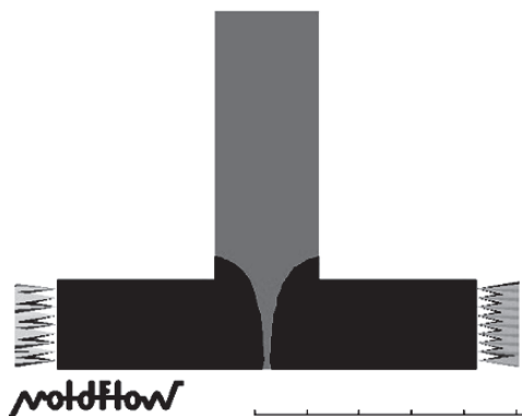
Fig. 2-4 Simulation by MPI software (Autodesk (C) ), front joining in mold cavity of shape \perp with opposite inlets
