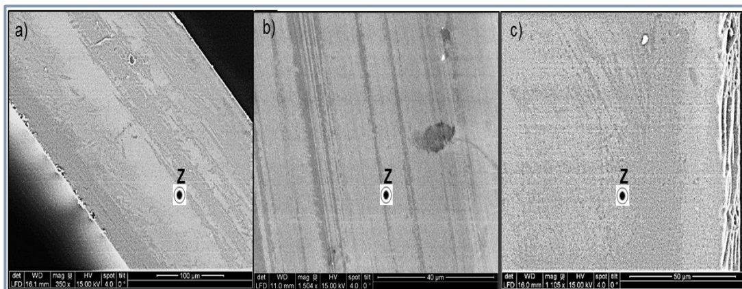
Fig. 3. 13 SEM images of cross sections of 42\text{ RY-LT} crystals etched with concentrated HF for 1 h: 42\text{ RY-CLT} crystal annealed at 750^\circ\text{C} (a), 42\text{ RY-NSLT} crystal with 49.8 mol% of \text{Li}_2\text{O} (b) and 42\text{ RY-subCLT} with 48.4 mol% of \text{Li}_2\text{O} (c) obtained by VTE treatment.
