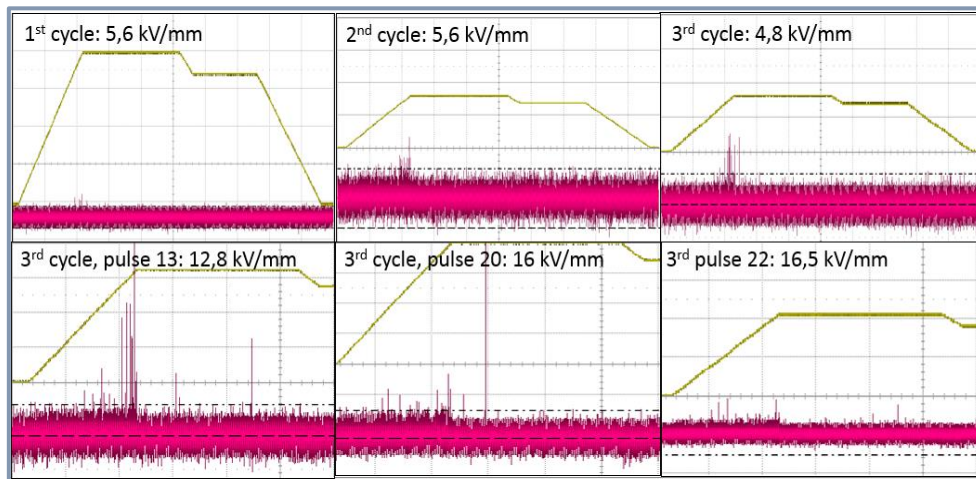
Fig. 3. 29 Transient current peaks observed during the poling of a 42 RY-NSLT:Fe (VTEN60) crystal
