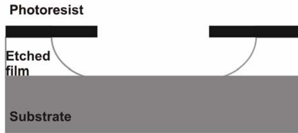
Fig.A2.6: Shape obtained after isotropic etching [Petersen 1982, Madou 2002, Józwik 2004 a]
