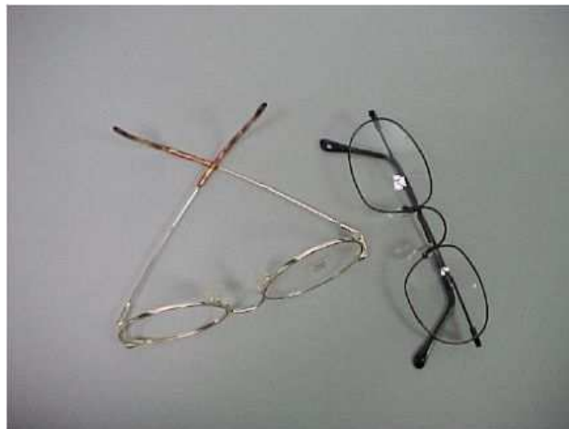
Figure I.10: Glass frames made of NiTi (Fig. 2 of Ref. [W&S])
