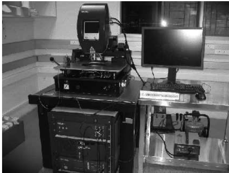
FIGURE 5.11 – MEMS Analyzer MSA-500 de la société Polytec.
