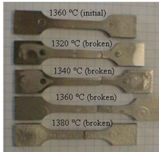
**Figure 3.23: Some of the tensile test specimens in 316L stainless steel sintered at different temperatures.**
