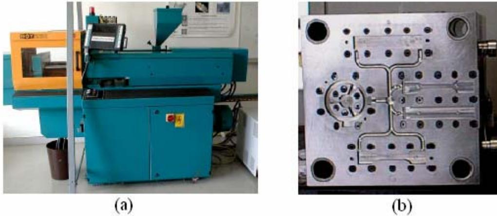
**Figure 3.3: Injection molding machine and the designed molds in the experiments [BAR 00].**
