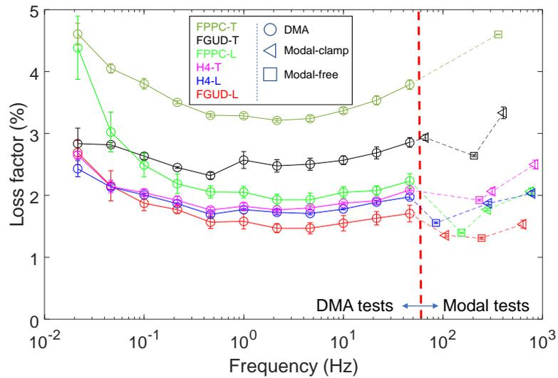
FIGURE III.20 – Loss factor in Modal and DMA tests. (Modal-clamp and modal-free refer to modal tests under free-clamped and free-free boundary conditions)
