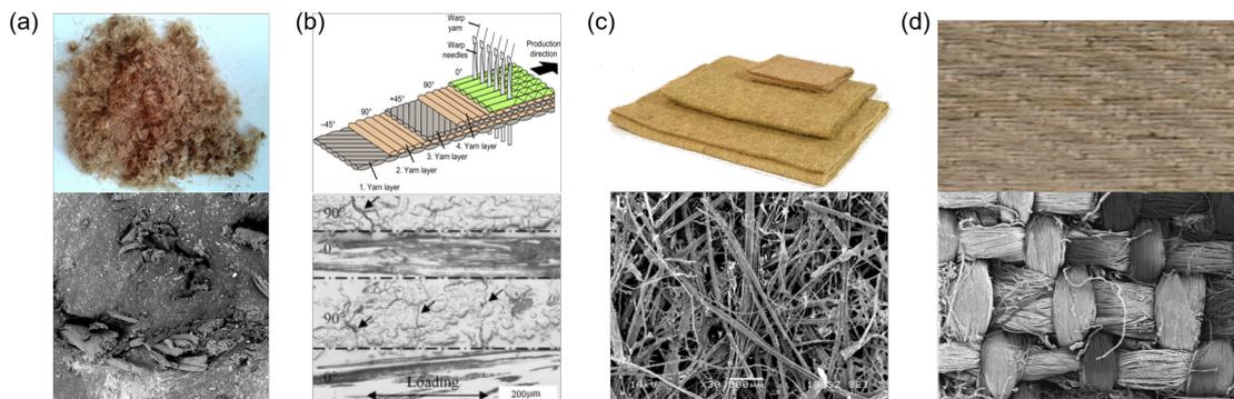
FIGURE 6 – Different reinforcements and micro-structures of (a) short fiber [Datta 17] (b) non-crimp [Schrank 17, Liang 14](c) non-woven [Reinders , Martin 16] and (d) woven fabric [Song 12, Corbin 20b]
