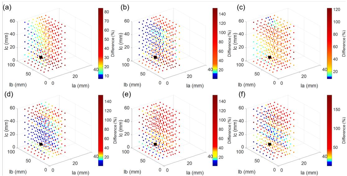
FIGURE III.10 – Difference of loss factor under various values of  $l_a$ ,  $l_b$  and  $l_c$  in modes 1-6 ((a)-(g)) (the blue points refer to difference (*err*) is less than 10 %, ■ refers to the final selected value)
