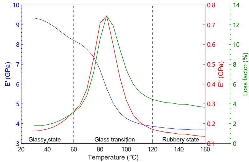
FIGURE II.2 – Typical dynamic mechanical properties of epoxy based composites
