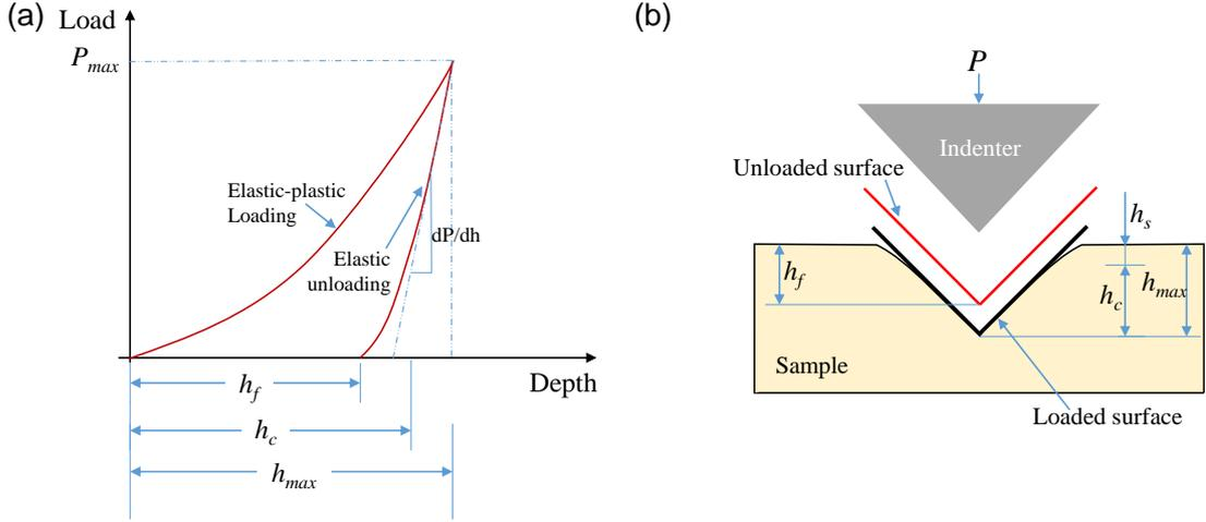
FIGURE IV.1 – (a) Typical loading-unloading curves ( $P_{max}$  is the maximum load during nanoindentation,  $h_f$  is the depth of the residual indentation,  $h_{max}$  is the depth from the original sample surface at load  $P_{max}$ ) (b) Profile change after indentation ( $h_s$  is the distance from the edge of the contact to the surface,  $h_s + h_c = h_{max}$ ,  $h_c$  is the contact depth measured from maximum depth  $h_{max}$ )
