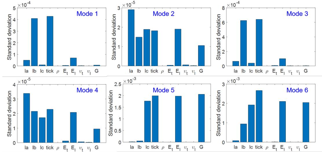
FIGURE III.11 – Standard deviation on loss factor obtained 5 % variation around the nominal value of the parameters in experimental setup (tick: thickness of the sample,  $\rho$ : density of the composites,  $E_t$  and  $E_l$ : Young’s modulus in transverse and longitudinal direction,  $v_t$  and  $v_l$ : Possion’s ratio in transverse and longitudinal direction, G: shear modulus)
