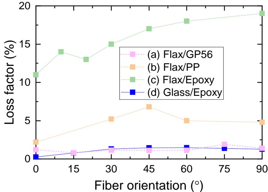
FIGURE I.4 – Variation of loss factor as function of fiber orientation in UD composites in longitudinal direction using modal tests (a) Flax/GP56, (b) Flax/PP, (c) Flax/Epoxy, (d) Glass/Epoxy [Daoud 17, Rueppel 17, Rahman 17b, Gao 11b]
