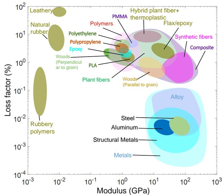
FIGURE I.1 – Ashby diagram: loss factor v.s. modulus at ambient temperature (summarized from refs.[Araújo 09, Duc 14b, Margem 10, Joseph 10, Jawaid 13, Towo 08, Saha 99, Mylsamy 11, Suresh Kumar 14, Sreenivasan 15, Ray 02, Pothan 03, Daoud 17, Shinoj 11, Karaduman 14, Mohanty 06, Etaati 14, Amenini 19, Mahmoudi 19, Li 17c, Ashworth 16, Cihan 19, Zhang 19, Essabir 13, El-Hafidi 17, Liang 10, Le Guen 16, Assarar 15, Rueppel 17, Madera-Santana 09, Mazuki 11])
