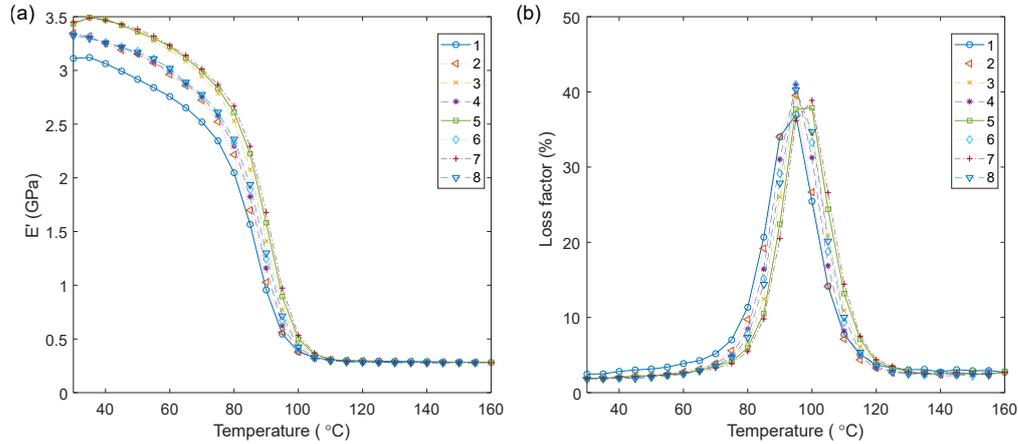
FIGURE II.13 – (a) Storage modulus and (b) loss factor of FGUD (post-curing at 130 °C and 1h) in transverse direction for each temperature cycles at 1 Hz
