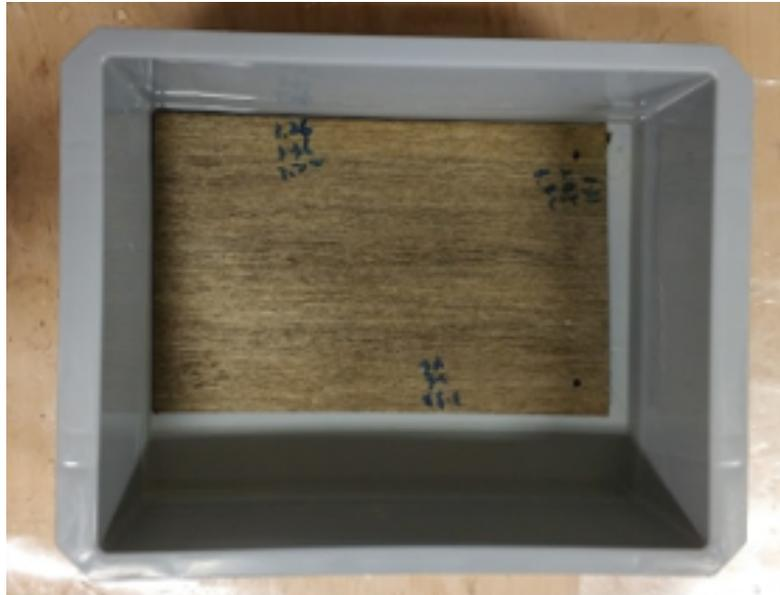
FIGURE III.5 – Water aging test at ambient temperature
