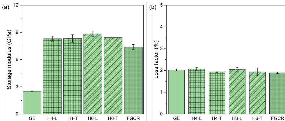
FIGURE II.18 – Comparison between balanced hemp fabric/GreenPoxly composites and FGCR in (a) storage modulus and (b) loss factor at 1 Hz and ambient temperature
