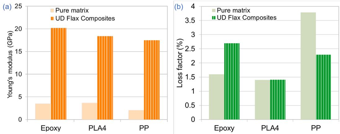
FIGURE I.6 – Young's modulus and loss factor of flax composites in the longitudinal direction and pure matrix measured by DMA at 1 Hz and ambient temperature (summarized from ref. [Duc 14b])
