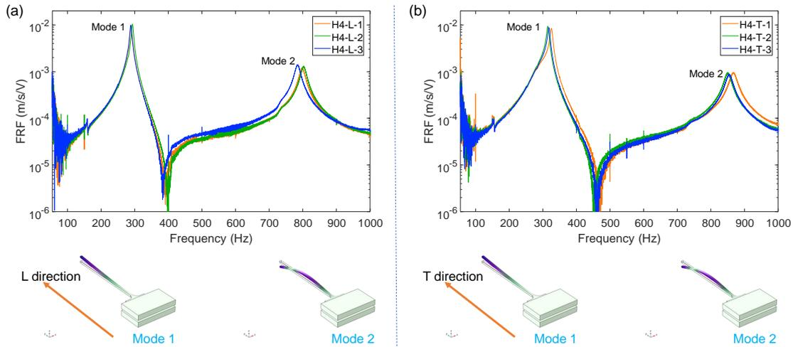
FIGURE III.18 – Modal response of H4 in (a) longitudinal direction, and (b) transverse direction
