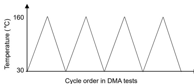
FIGURE II.12 – Temperature cycle during DMA test
