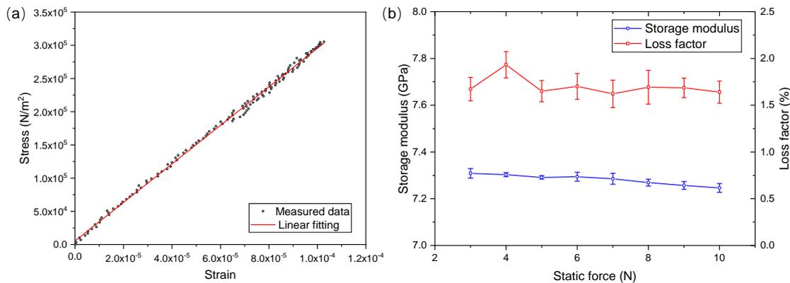
FIGURE II.6 – Verification of the excitation setup in DMA tests (a) Response of stress-strain under quasi-static tension (b) Storage modulus and loss factor with different static and dynamic forces under tension mode
