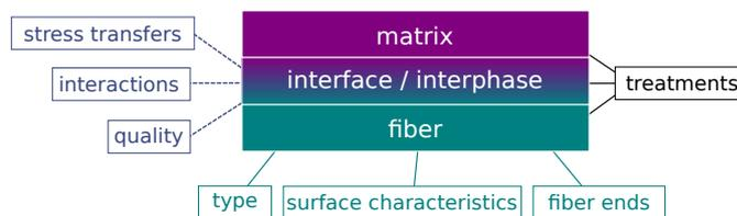
FIGURE I.7 – Parameters related to the interface properties
