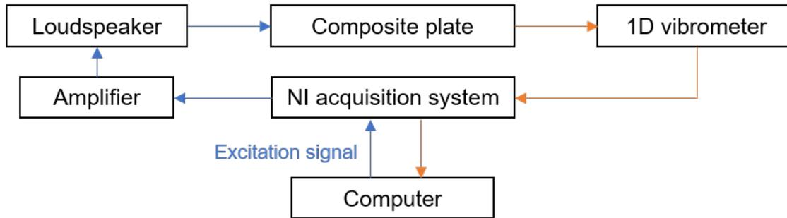
FIGURE III.4 – Schematic diagram of the experimental system
