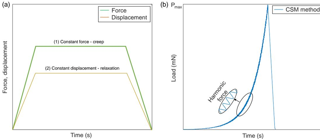
FIGURE IV.2 – Protocols for viscoelastic properties measurement from (a) creep and relaxation tests (b) CSM method
