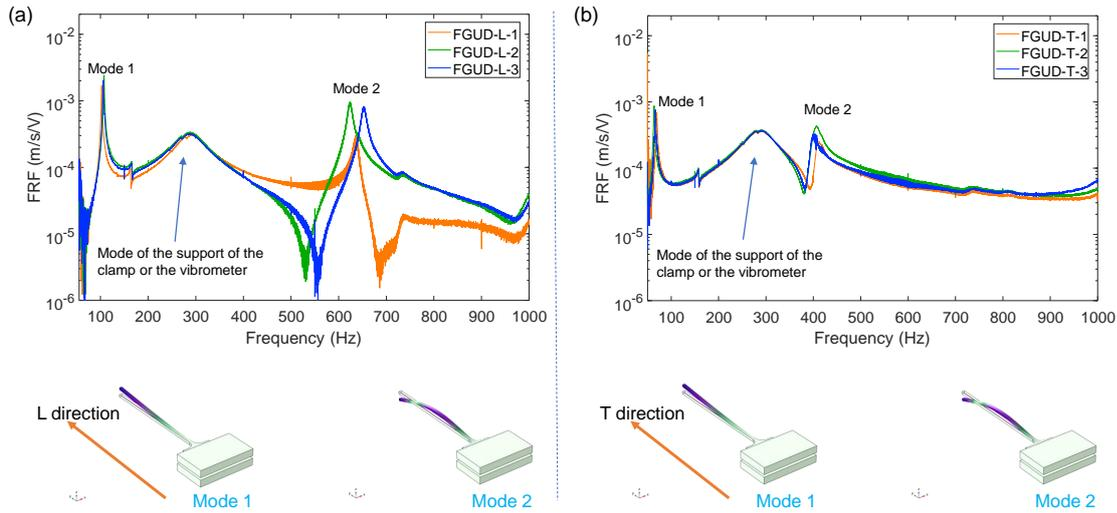
FIGURE III.16 – Modal response of FGUD in (a) longitudinal direction, and (b) transverse direction
