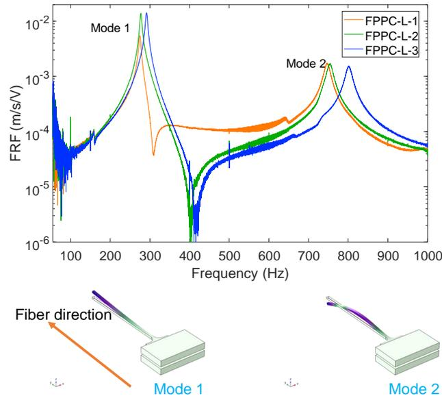
FIGURE III.17 – Modal response of FPPC in longitudinal direction
