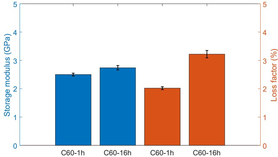
FIGURE II.14 – Comparison of storage modulus and loss factor of pure GreenPoxy at 1 Hz and ambient temperature using the optimized curing time and the datasheet from Sicomin<sup>®</sup> (C60-1h refers to sample curing at 60 °C and 1 hour with post-curing at 130 °C and 1 hour, C60-16h refers to sample curing at 60 °C and 16 hour with post-curing at 100 °C and 1 hour)
