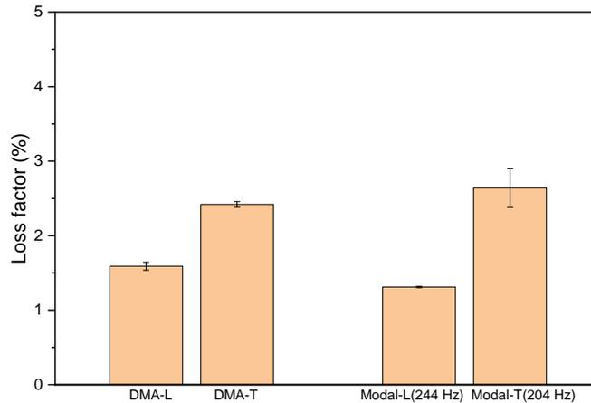
FIGURE III.13 – Comparison of the loss factor values determined for FUGD material in DMA and modal tests. (The results from DMA test is at 1 Hz and modal tests are obtained from the flexural modes in longitudinal direction (around 244 Hz) and transverse direction (204 Hz))
