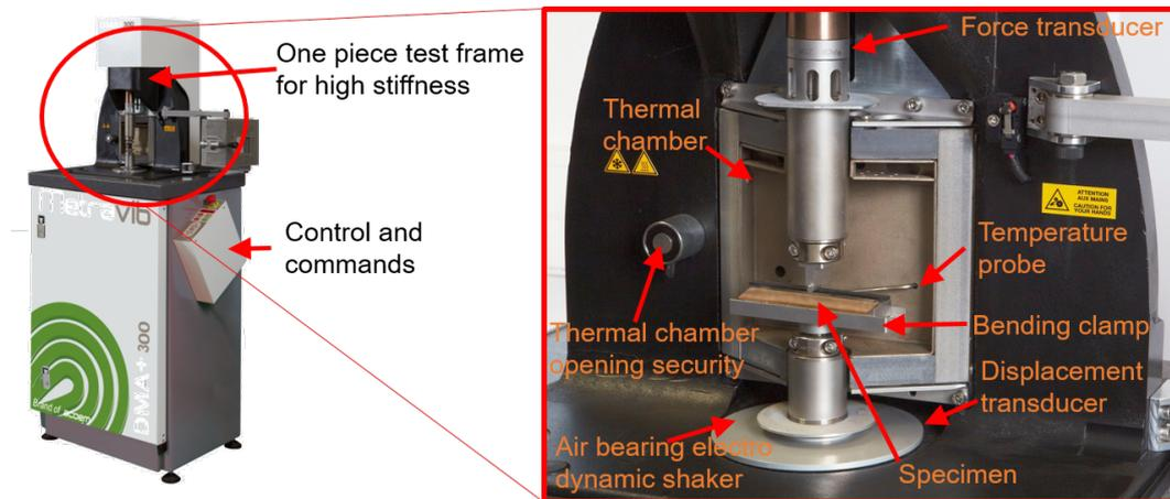
FIGURE II.3 – Main assets in Metravib<sup>®</sup> DMA+300
