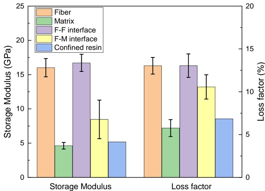
FIGURE IV.18 – Storage modulus and loss factor in each component using CSM method at 5 Hz (single point in confined zone without errorbar)
