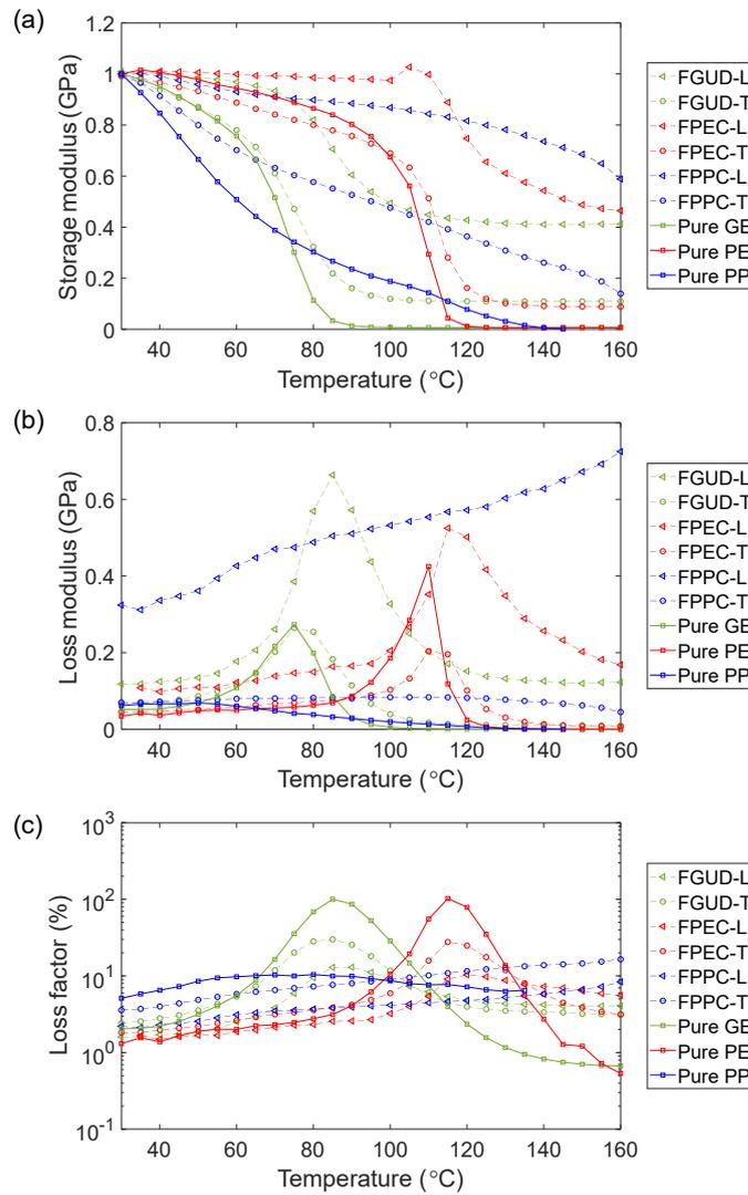
FIGURE II.20 – (a) Normalized storage modulus, (b) loss modulus, (c) loss factor of FFRC and pure matrix at 1 Hz and 30 - 160 °C
