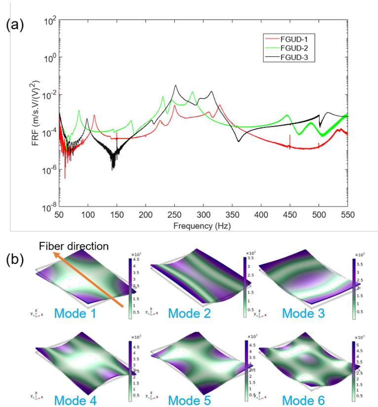
FIGURE III.12 – (a) FRF results of numerical model and experiment, and (b) modal shape simulated by numerical model for FGUD in free-free conditions
