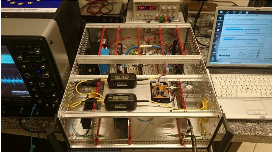
Figure 3.1: Picture of the photonic RC setup based on an EO phase delay dynamics.
