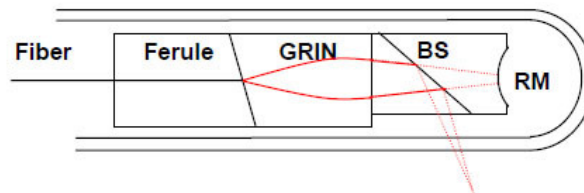
Figure 2.20: Schematic of the probe designed by Tumlinson et al. [84]. BS: beam splitter; RM: reference mirror; GRIN: gradient index.
