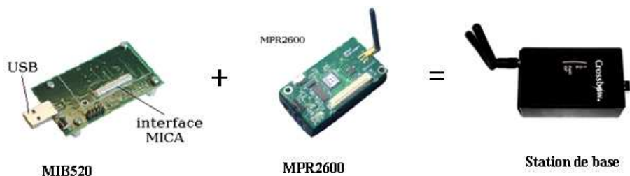
Fig A.6- Station de base
