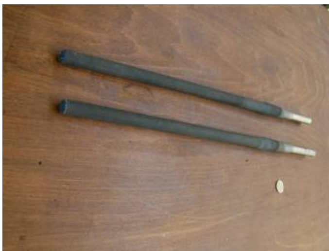
Figure 11: Photo of the thermal-sprayed solid oxide fuel cells (after H 2 reduction and without cathode layer).
